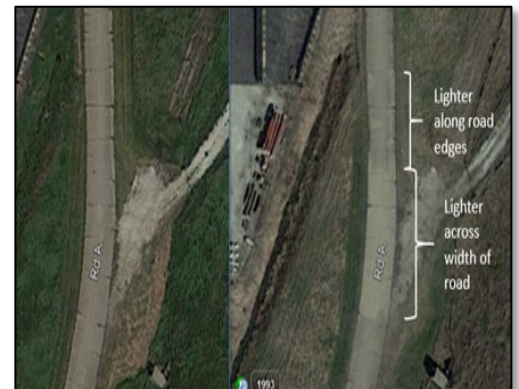
Lighter area of the road likely indicates where the foam flow occurred.
