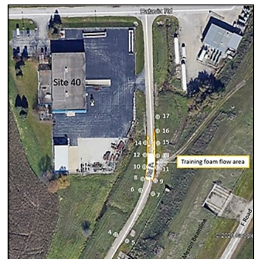
Location of surface soil samples collected in December 2023; analytical results indicate an area of PFAS contamination on both sides of the road.
