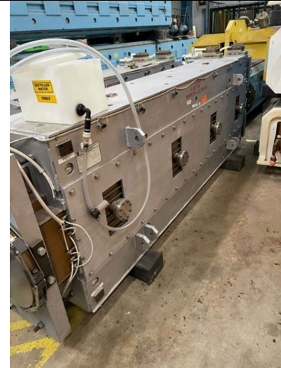
Magnet stored on non-rated plastic lumber in single layer - acceptable
