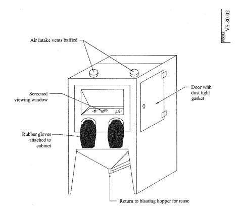
An abrasive blast cabinet is an enclosure in which the blast is directed by an operator located outside of the cabinet. Air contamination is controlled primarily by enclosure although more abrasive blast cabinets have powered exhaust systems. See also "Abrasive Blast Booth" above.
