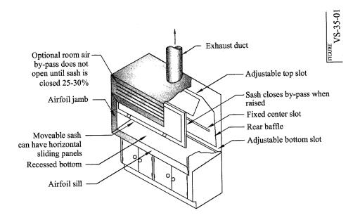
Laboratory hoods are power-ventilated enclosures with transparent sliding doors. They are typically employed in laboratory environments in which atmospheric hazards are variable and generally unquantified.
