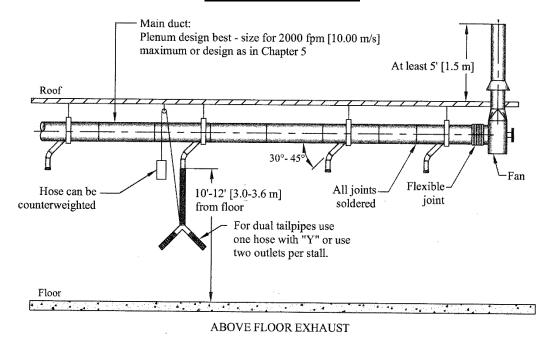
Vehicle exhaust systems are used to control air contaminants from vehicle engines.
