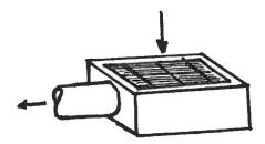
A downdraft table is used to control air contaminants generated in welding and cutting operations.
