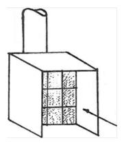
A paint booth is a power-ventilated, usually box-shaped enclosure which is open on one side. It is used to control atmospheric contaminants generated in spray coating operations. Spraying should be confined to the inside of the booth.
