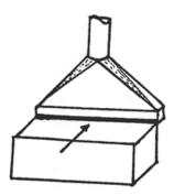
Slot exhaust systems are used to control vapors or gases from extended sources of contamination such as long tanks or tables. They are typically used for dip tanks, degreasing, or soldering operations. Air enters the system via a horizontal slot(s) situated along one, or both, long edges of the source. The performance of slot exhaust systems is maximized by minimizing the slot-towork distance and enclosing the system as much as possible.
